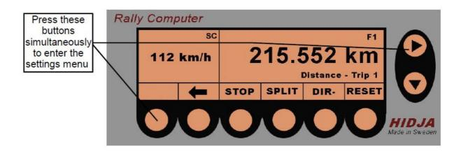
All calibrations and installations can be interrupted by pressing **BACK**. Some functions in the smaller windows does not get updated when the setup menu is active.
