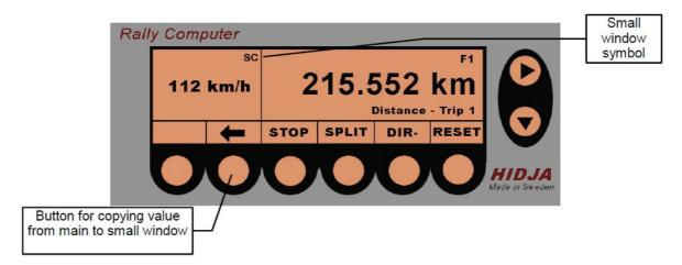
One press on the arrow button copies the current records from the main window to the smaller window. When a record have been copied from the main window to a smaller, an explanation symbol will appear to the right of the smaller window.
