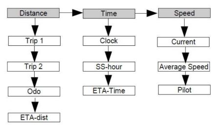
The menu consists of one main menu and several sub menus. The main menu consists of: *Distance, Time, Speed.* There are a number of different sub menus below every main menu alternative. You can for instance find *average speed* and *speed limit* as sub menus to *Speed* etc.
